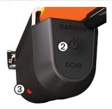
The red LED ③ flashes (single blink) when the DC 40 is on and searching for satellite signals.
